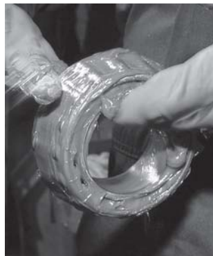
Fig. 23. Grease can easily be packed by hand.
